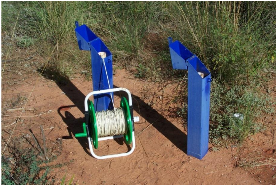
Electronic depth meter used for groundwater level measurements
