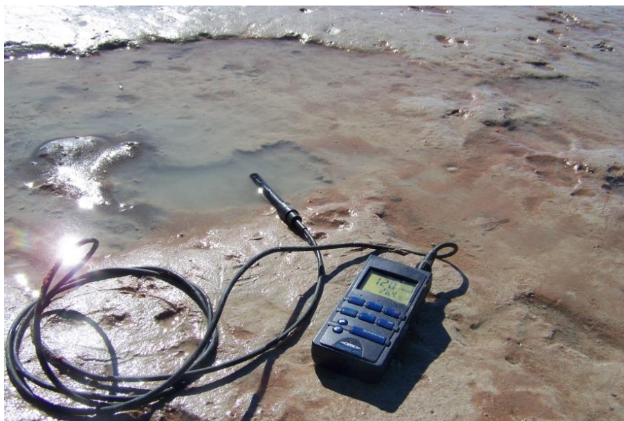
Apparatus set up for fresh water discharge delineation through the Town Beach intertidal zone
