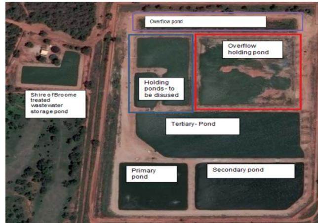
The two year lag and late start to reline seeping ponds is concerning, with an early wet forecast (80%) and no plans to reline the Secondary, Tertiary (lined 1982 with compacted pindan) or Primary ponds (Relined 2004 with geotextile - old technology). RBWG are urging Water Corp to install 'world best practice' liners in all ponds to prevent further seepage.
